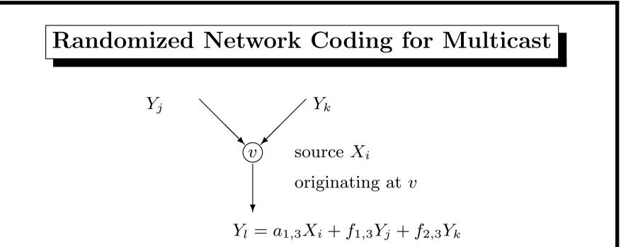
Determining feasibility: min-cut max-flow bound satisfied for each receiver [ACLY00]
