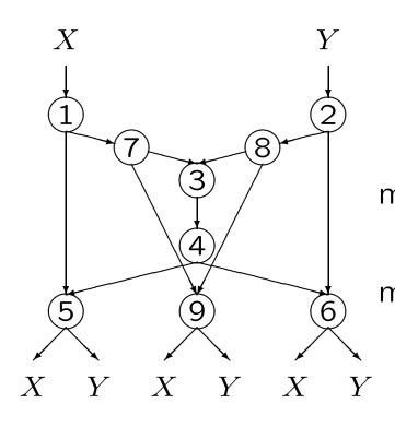
$$\begin{split} \min\{C_{17}, C_{73}, C_{34}, C_{46}, C_{79}, C_{15} + C_{45}\} \\ &\geq H(X|Y) \\ \min\{C_{28}, C_{83}, C_{34}, C_{45}, C_{89}, C_{26} + C_{46}\} \\ &\geq H(Y|X) \\ \min\{C_{15} + \min\{C_{17}, C_{73}\} + \min\{C_{28}, C_{83}\}, \\ &C_{15} + C_{34}, C_{15} + C_{45}\} \geq H(X,Y) \\ \min\{\min\{C_{17}, C_{73}\} + \min\{C_{28}, C_{83}\} + C_{26}, \\ &C_{34} + C_{26}, C_{46} + C_{26}\} \geq H(X,Y) \\ \min\{C_{17}, C_{79}\} + \min\{C_{28}, C_{89}\} \end{split}$$
