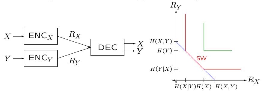
Optimal error exponents achievable with: Linear encoders and minimal entropy decoders or maximal a posteriori probability decoders achieve optimal performance.
