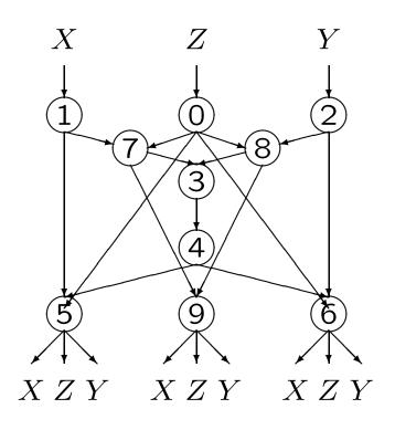
min cut from  $X \ge H(X|Y,Z)$ min cut from  $Y \ge H(Y|X,Z)$ min cut from  $Z \ge H(Z|X,Y)$
