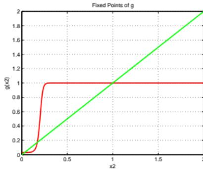
Theorem: If  $g$  has no degenerate fixed points,  $\exists$  odd number of equilibria  $u^1, u^2, \dots, u^{2m+1}$  indexed by increasing values of  $x_2$ .  $u_{2i+1}$  are stable,  $u_{2i}$  are unstable. If  $B(u_i)$  denotes the basin of attraction of  $u_i$ , then
