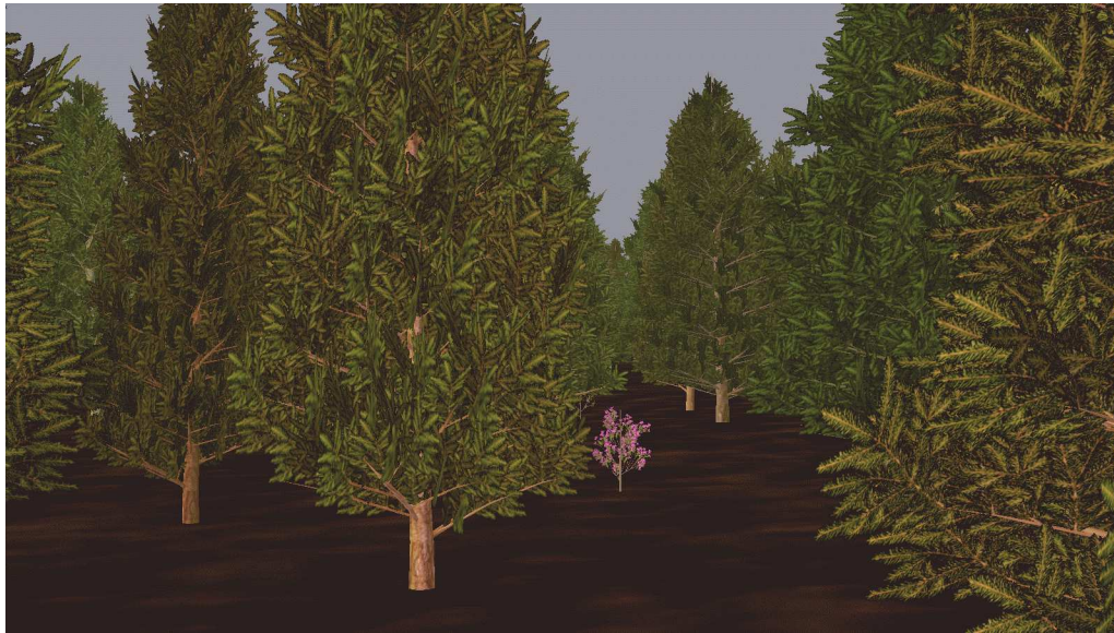
Figure 4: A frame from a flythrough of a forest scene accelerated using visible zone maintenance. The scene consists of 835,089 tree objects, and 10 billion total polygons. For this frame, 50 trees and 1,887,714 polygons were rendered. The rendering time was 85 ms., while the time devoted to visibility maintenance was 6 ms.
