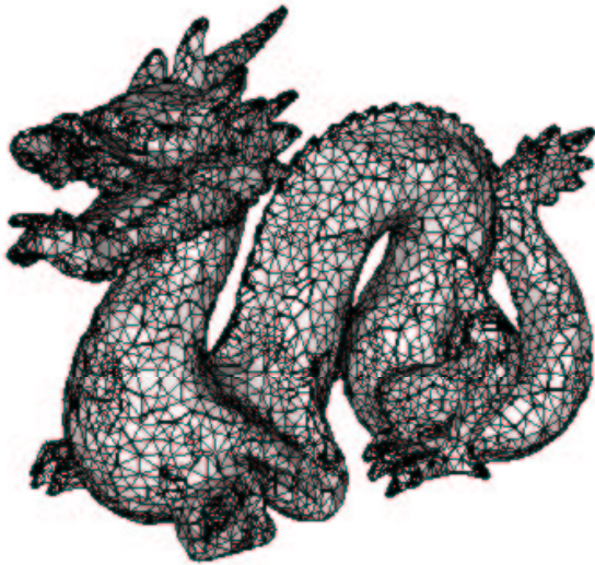
Figure 15. Dragon is decimated such that its original edge length scale is reduced by 8 times. The mesh consists of ~11K vertices, 34K edges and ~22K faces.
