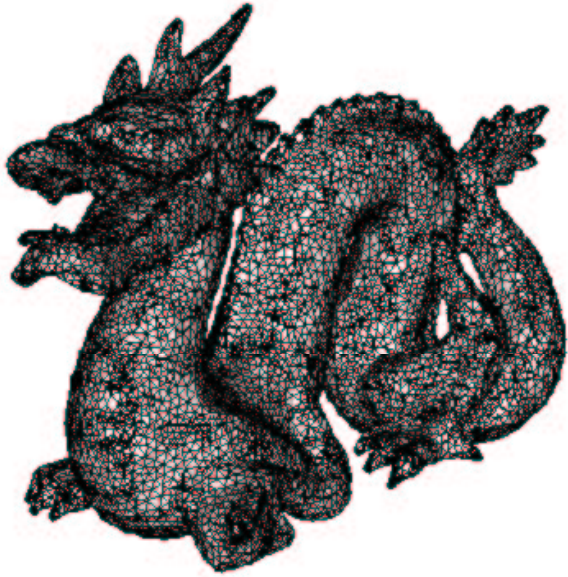
Figure 14. Dragon is decimated such that its original edge length scale is reduced by 4 times. The mesh consists of ~22K vertices, 66K edges and ~44K faces.
