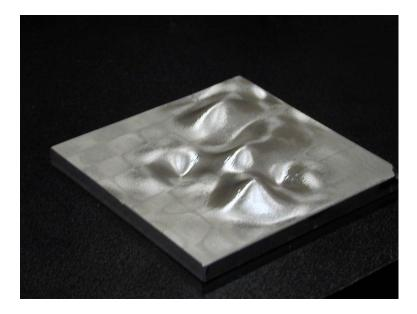
Figure 9: Machined surface using 0.25in diameter cutter
