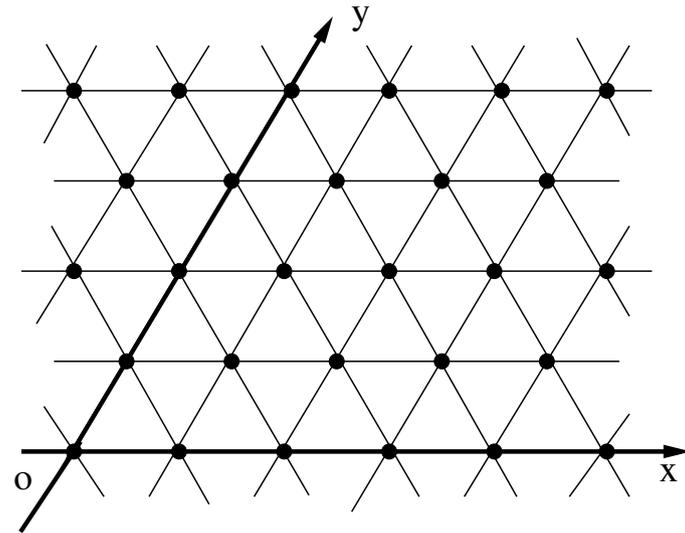
A Network of Transmitters with a Hexagonal Cell Covering
