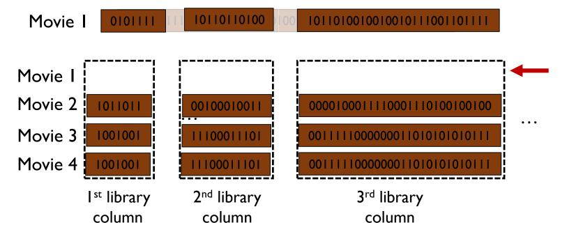
Narrow first column => small startup delay
