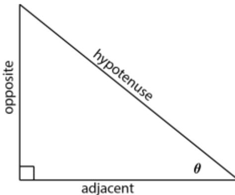
Figure 5: Right triangle with opposite, adjacent and hypotenuse labeled
