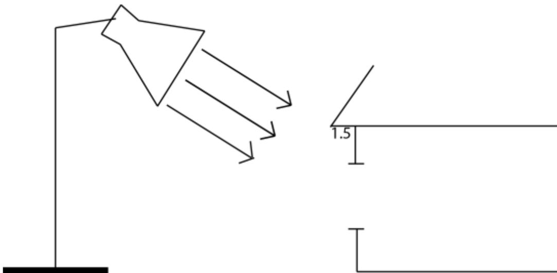
Figure 14: Heat lamp at about a 30° angle with the window
