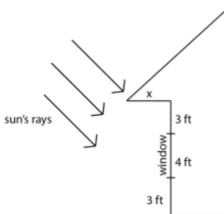
Figure 13: Demonstrates how an overhang can block the sun's rays
