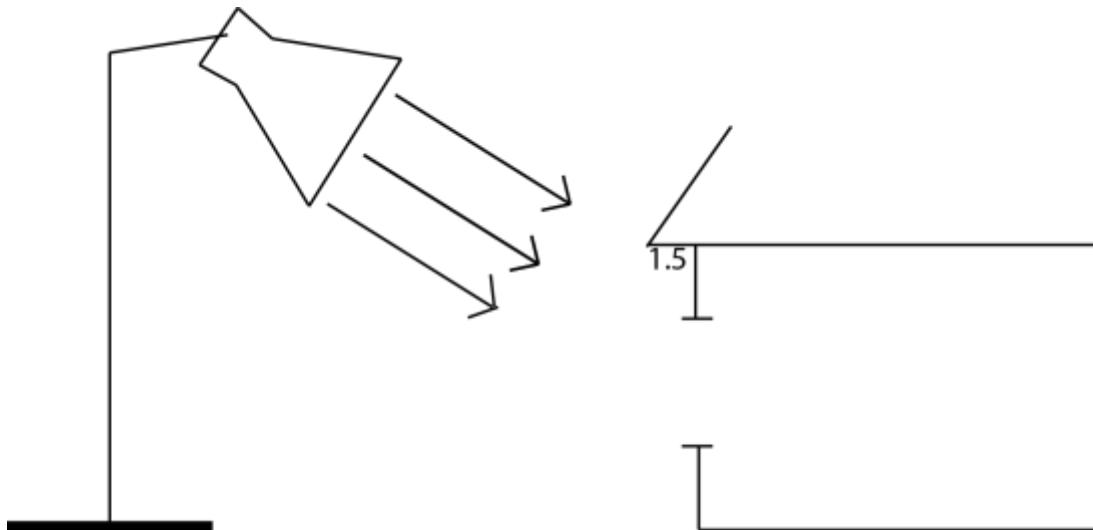
Figure 14: Heat lamp at about a  $30^\circ$  angle with the window
