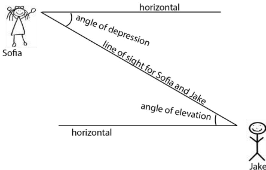
Figure 6: Illustration of angle of depression and angle of elevation
