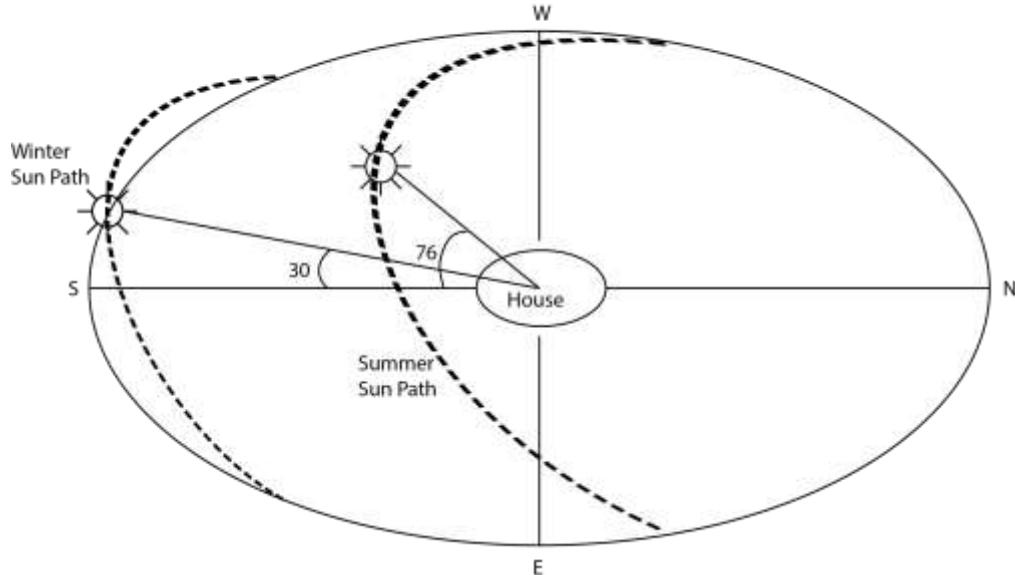
Figure 11: Angles of elevation of the sun's rays at noon during winter ( $30^\circ$ ) and summer ( $76^\circ$ ) for Vilas, NC (<http://www.susdesign.com/sunangle/>)
