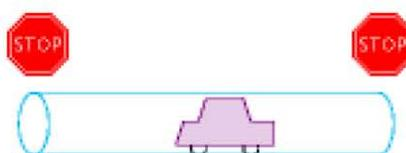
Braking is not the only way for energy-loss to occur. Another way that a moving car consumes energy is by making air swirl around it as it moves. When moving, a car pushes air out of its way, creating a tube of swirling air behind it, which moves at a speed close to  $v$ . Since this tube of air is moving, it possesses kinetic energy as well.
