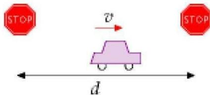
Any moving car has a certain amount of energy of motion associated with it. This is the minimum amount of energy that it took to bring it to this speed, and also the amount of energy you would need to dissipate in stopping the car.
