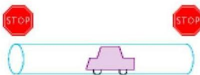
Braking is not the only way for energy-loss to occur. Another way that a moving car consumes energy is by making air swirl around it as it moves. When moving, a car pushes air out of its way, creating a volume of swirling air behind it, which moves at a speed close to  $v$ . Since this displaced air is moving, it possesses kinetic energy as well.
